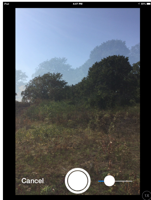
Figure 2. The ghost image feature allows the user to line up the current photo with the previous photo. This feature ensures that the new image is taken in the same place and position as before, so a consistent photographic record can be maintained.
