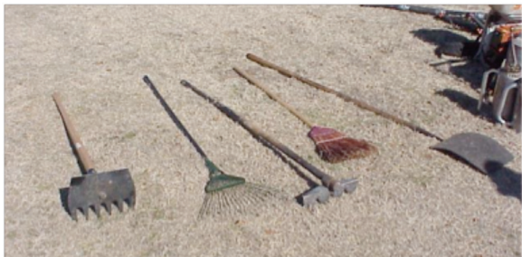
Common handtools used on prescribed burns, from left to right: McLeod, leaf rake, fire rake, broom and swatter.
